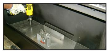
Figure 16.5 Remove Valve Plate Screws
